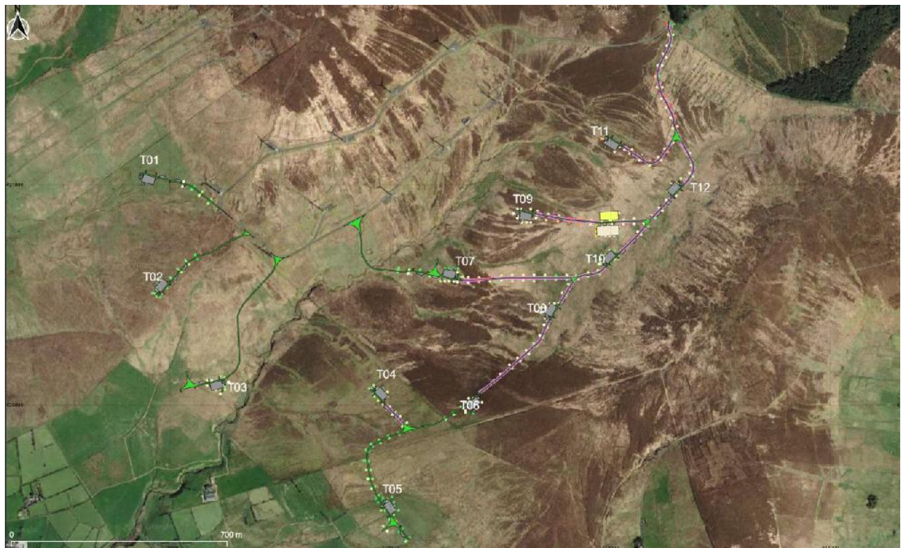
Figure 3.2: Extract Figure A1 – Peat Depth Map – Purple track sections indicate floating type
