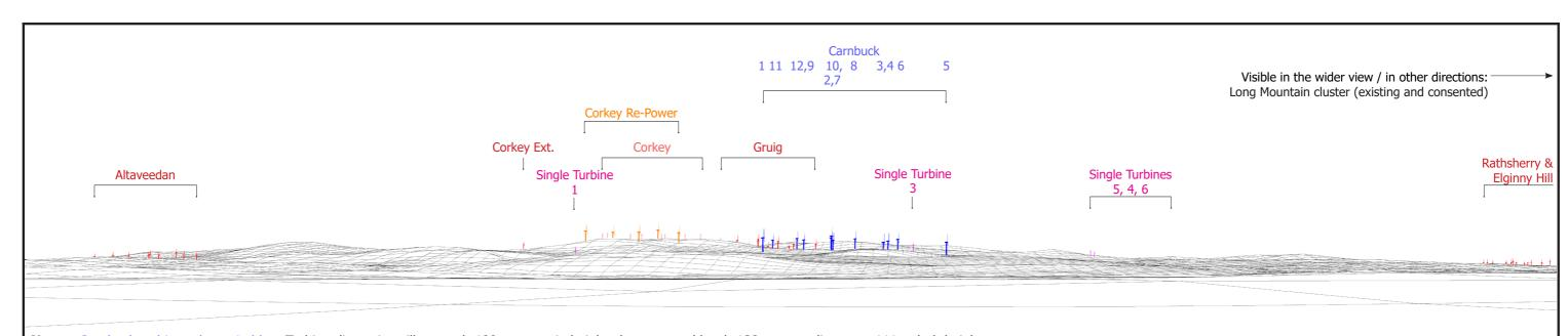
Notes: Carnbuck turbines shown in blue. Turbine dimensions illustrated: 180 m max. tip height above ground level; 138 m rotor diameter; 111 m hub height
