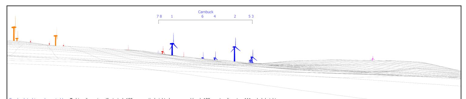
Carnbuck turbines shown in blue. Turbine dimensions illustrated: 180 m max. tip height above ground level; 138 m rotor diameter; 111 m hub height
