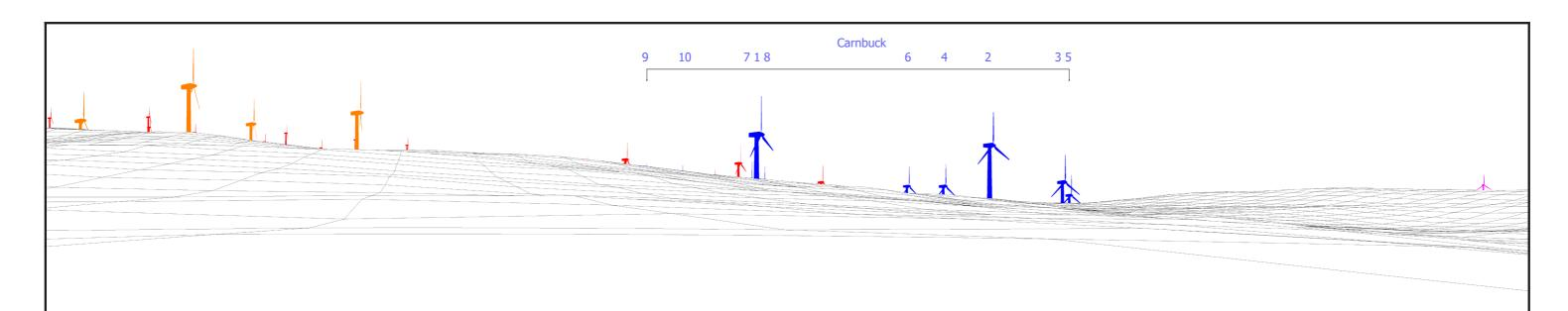
Carnbuck turbines shown in blue. Turbine dimensions illustrated: 180 m max. tip height above ground level; 138 m rotor diameter; 111 m hub height
